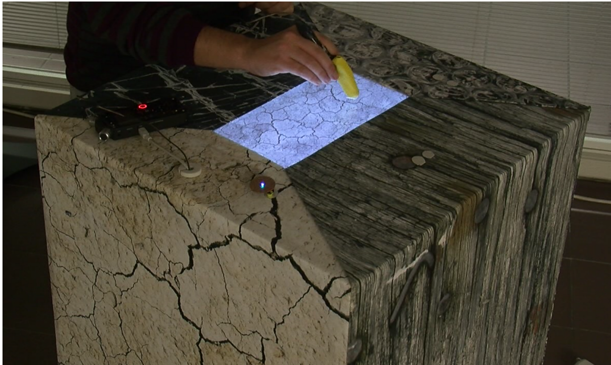
Figure 9: Installation configuration of Sketch-a-Scratch: Top of the installation with tablet, stylus and audio recorder. The rounded token with the red led allows to browse and switch between the four textures.
